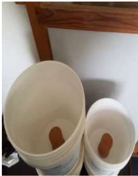
Silver coated candle filter and its candle
